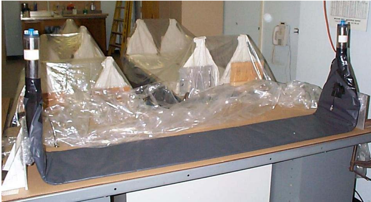
Figure 7: A TCD detector module being prepared for testing. The active section of detector is the long flat section. The adiabatic lightpipes make a 90° bend, and carry the light to the photomultipliers. The detector is wrapped in aluminum foil covered with DuPont Tedlar. Additional modules can be seen in the background.
